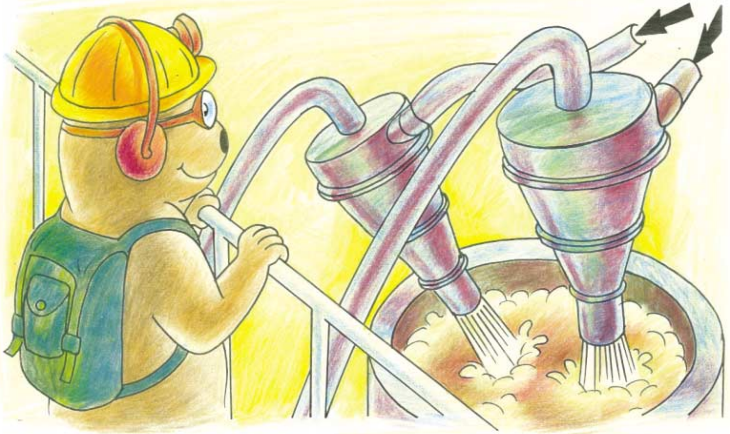
Hydro-cyclones swirl a muddy mixture of powdered ore and water into small tornadoes to separate heavy minerals from light waste rock.
