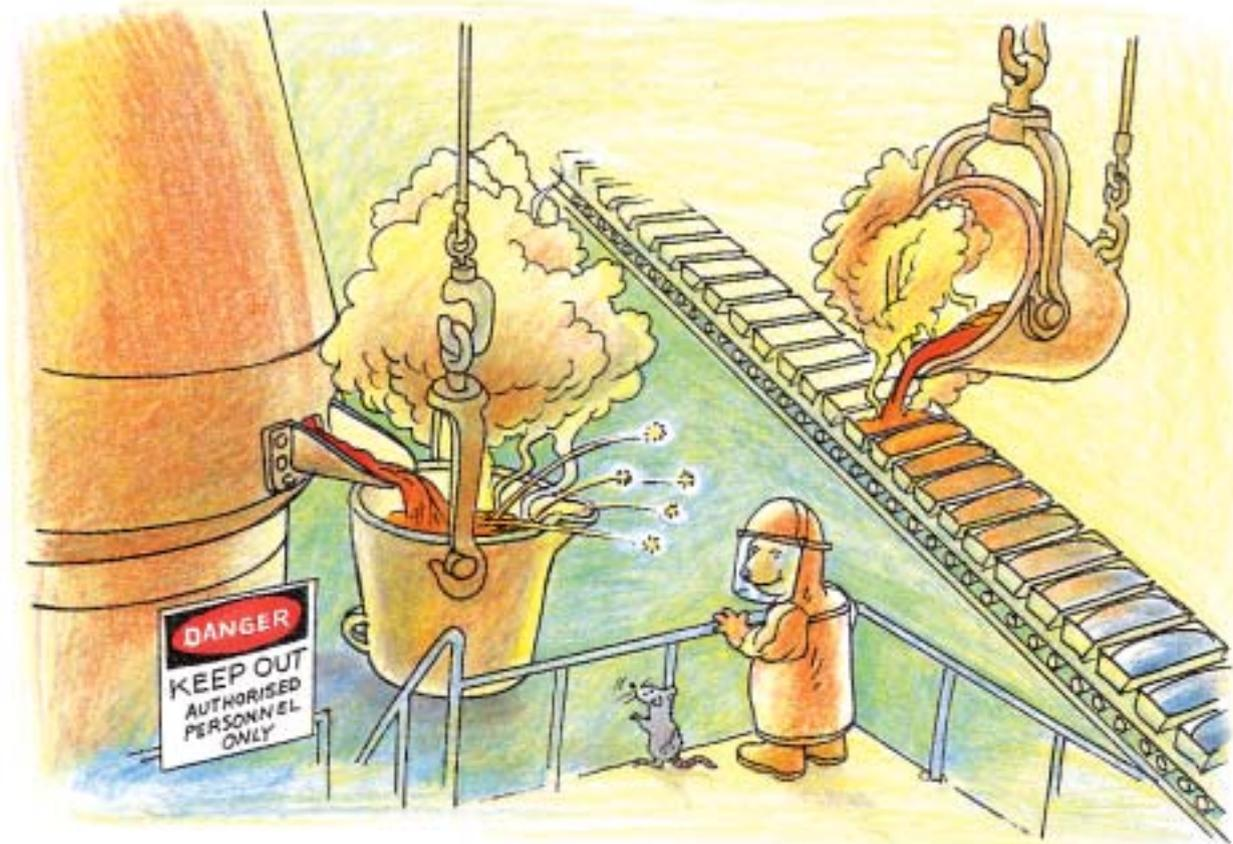
Several times a day the furnace is “tapped”. A hole is opened at the bottom of the furnace. Molten metal flows into a LADLE. The metal is then poured into special moulds. It cools to form solid INGOTS. 13
